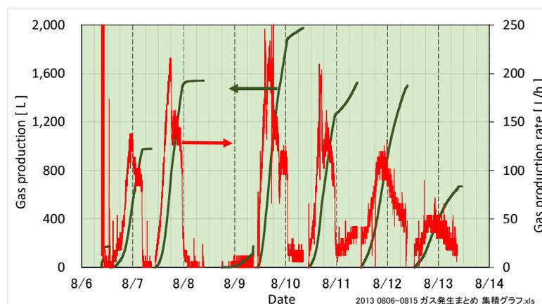
Fig. 2. Results of the workout of the pilot plant by fed batch operation with molasses.
