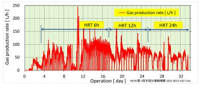
Fig. 4. Gas production rates at each HRT operation.
