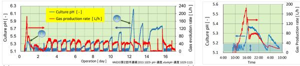
(a) The second operation by the newly found microflora.(b) The detail drawing of mark 1.Fig. 5. Culture pH rising appeared at fed batch operation by the newly found microflora.
