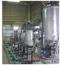
Photo 1. Small pilot plant set at Itoman city in Okinawa. The top tank is the fermentor with 200L volume.
