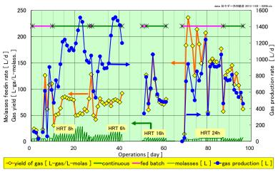
Fig.3. Results of continuous operations by the HN001.
