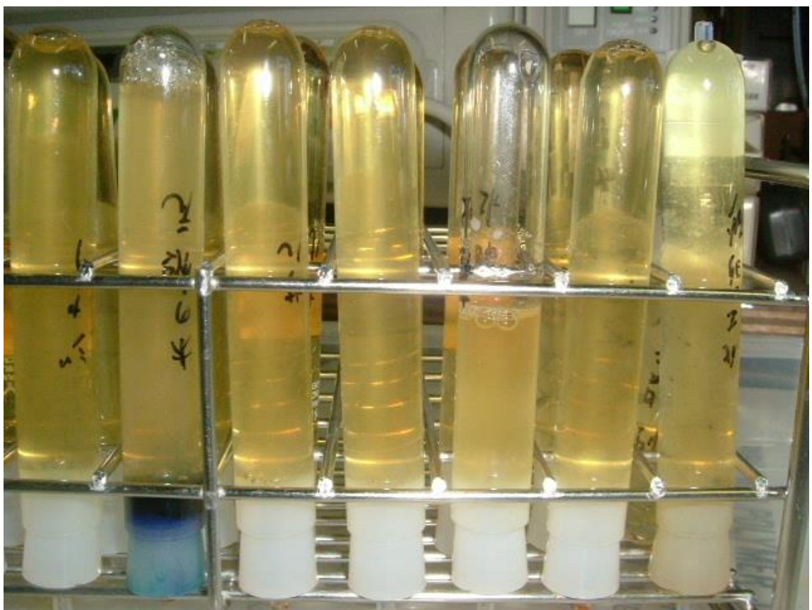
Fig.2.1. A picture of screening. There is a hole 2mm in diameter on silicon plug. If bacteria produce gases, culture medium is detruded.
